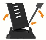
**NOTE:** Make sure the band is secure. The watch pin should align with the holes on the device.
