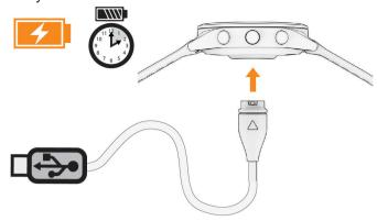
2 Plug the other end of the cable into a USB charging port.
