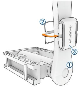
4 Rotate the crank arm to check for clearance. The sensor and bands should not contact any part of your bike or shoe.
