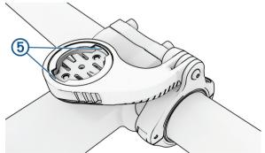
**9** Press down slightly and turn the Edge device clockwise until it locks into place.
