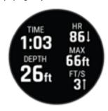
**In-dive screen:** Displays the information about the current dive, including the elapsed time, current and maximum depth, heart rate data, and rate ascent or descent.
