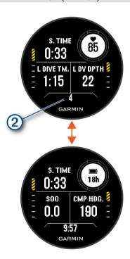
Surface interval screen: Displays the current surface interval time, as well as the elapsed time, maximum depth, and temperature for your last apnea dive. You can edit the data fields.
