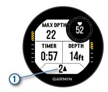
**In-dive screen:** Displays the information about the current dive, including the elapsed time, current and maximum depth, heart rate data, and rate of ascent or descent. You can edit three of the data fields (*Customizing the Data Screens, page 21*).
