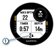
In-dive screen: Displays the information about the current dive, including the elapsed time, current and maximum depth, heart rate data, and rate ascent or descent. You can edit three of the data fields (Customizing the Data Screens, page 21).
