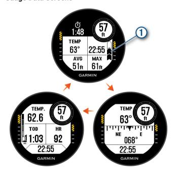
**Dive stopwatch:** Displays the bottom time stopwatch, average depth, maximum depth, and rate of ascent (*Using the Gauge Dive Stopwatch, page 9*).
